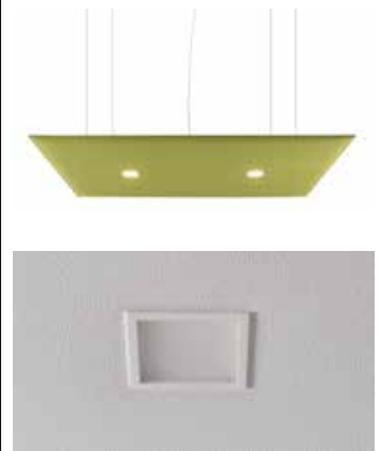
Description: Fixture complete with a high efficiency LED light source with a nominal luminous flux of 2200 lm (3000 K). Structure made from steel. Recessed light made from epoxy polyester powder coated aluminium and equipped with an opal polycarbonate diffuser and driver. Electrical cable length 390 cm included. Its degree of protection against the penetration of dust, solid objects and liquids is IP40.
