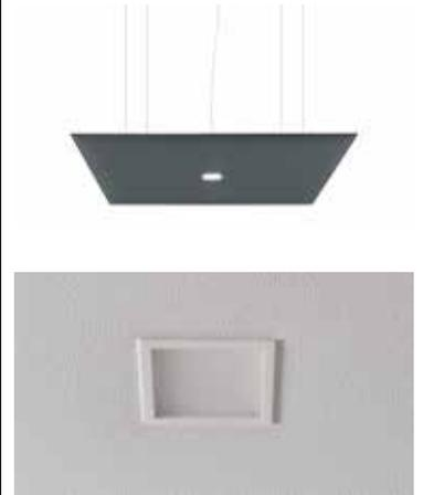
Description: Fixture made from epoxy powder coated steel and equipped with two drivers. Suitable for housing two recessed lights provided with a high efficiency LED light source with nominal flux 1440 lm (3000 K). Electrical cable length 390 cm included. Its degree of protection against the penetration of dust, solid objects and liquids is IP43.
